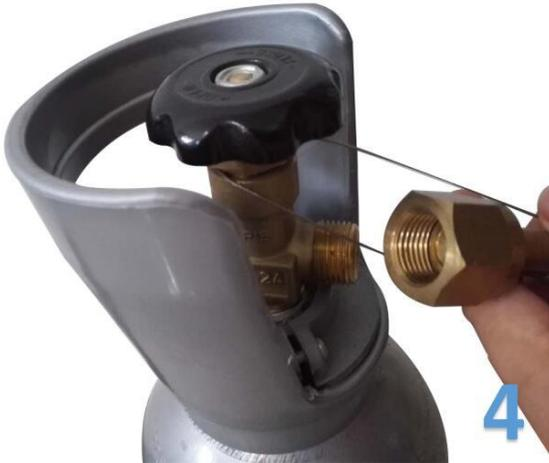
Hang the steel wire on the valve to keep safe.
