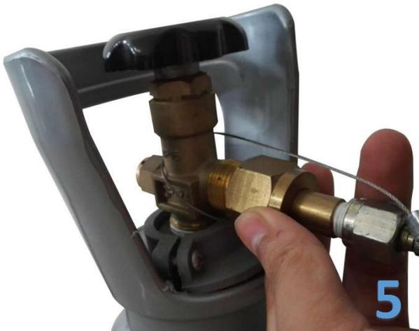
Put a rubber sealing ring in the nut of the dry ice maker and then connect the nut to the CO2 cylinder, use your fingers to screw tight until you can't screw.
