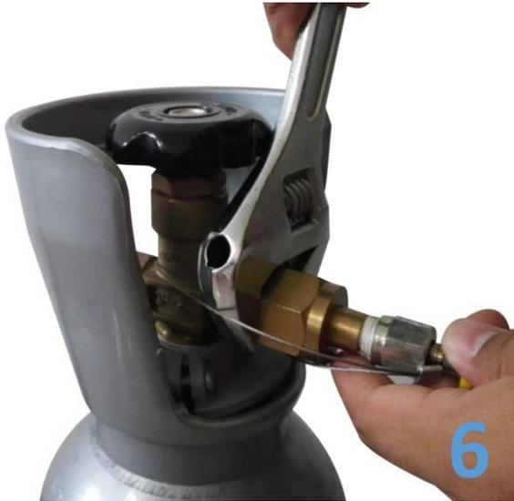
Use a wrench to reinforce the connection of the nut and the valve.
